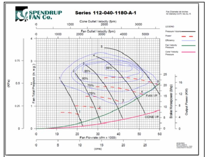
Figure 5. Booster Fan Characteristics Curve.
