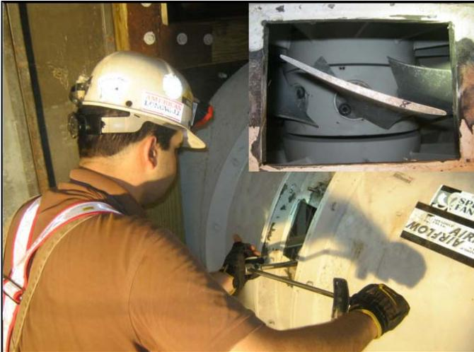
**Figure 6.** Adjusting blade settings.
