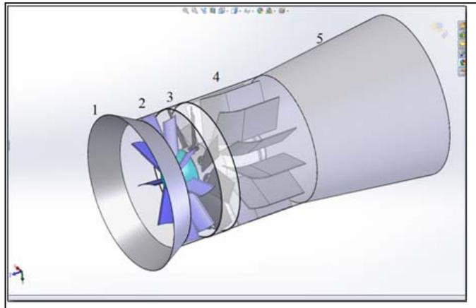
Figure 10. The geometric model of MS&T Booster fan.
