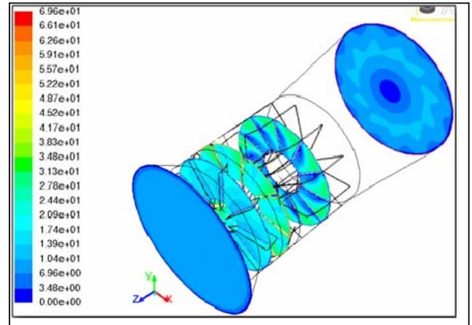
Figure 15. Velocity magnitude (m/s) distributions at various cross-sectional planes.
