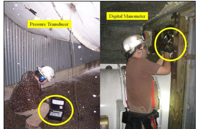
Figure 4. Pressure Measurements across the Bulkhead.
